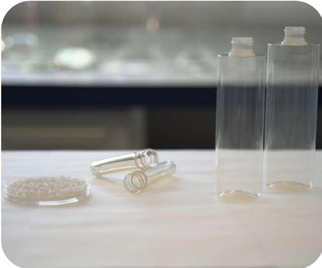
We currently have PLA-Premium grades, aimed at different industrial extrusion and injection applications.
